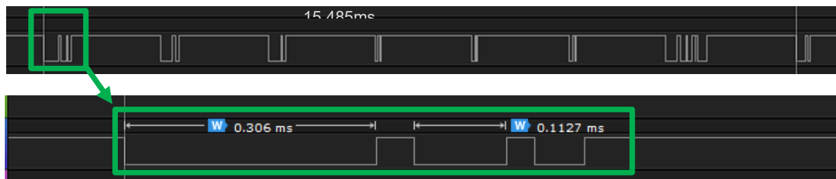
Figure 15. High-Duty Cycle Wi-Fi TX Active
