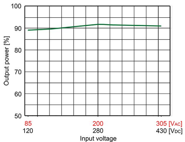
PAC30D12BS3 Efficiency vs input voltage at full load
