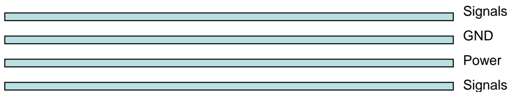
Figure 14: Typical 4-layer PCB construction
