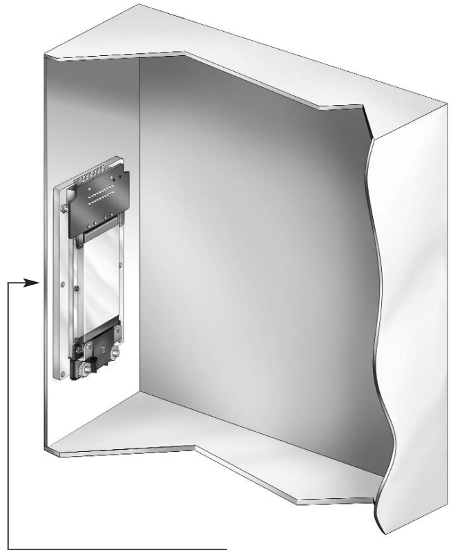
VIPAC Array mounted to cabinet wall with thermal compound between VIPAC Array and cabinet wall.
