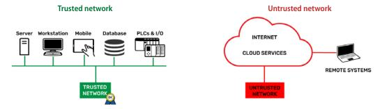
groov EPIC is not a router, which functions to join two networks together. Instead, groov EPIC keeps your trusted network isolated from your untrusted network by **not routing** network traffic **between** its network interfaces.
