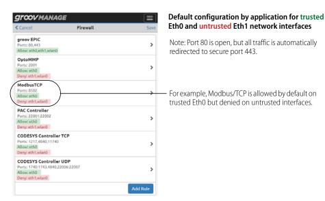
Remember that the default configuration assumes that ETH0 is on a trusted network. Make sure that network actually is trusted.
