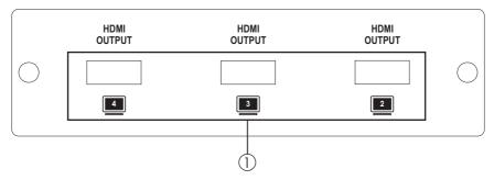
(1) HDMI OUTPUT 2/3/4: Connect each of the output ports to an HDMI display. When more than one output source is connected, an identical video signal will be shown on the connected displays.
