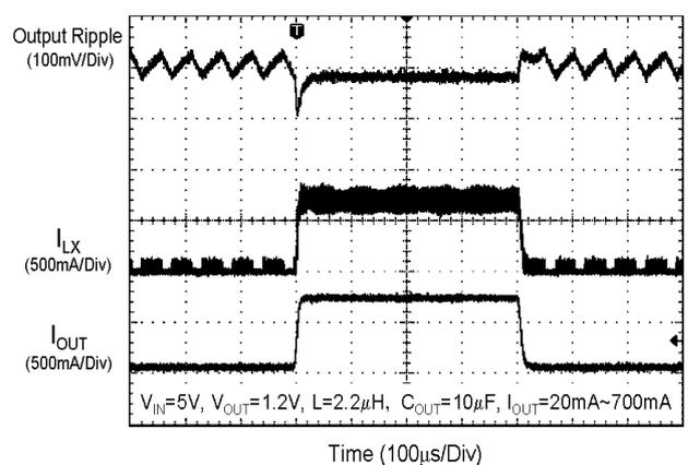
Fig. 14 Load Transient Response
