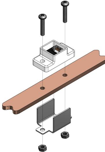
For the B version current sensor the upper half of the sensor is attached to the busbar using standard hardware. The lower half of the housing is then clipped to the upper half for a secure connection. The lower housing also serves as protection for the shield.
