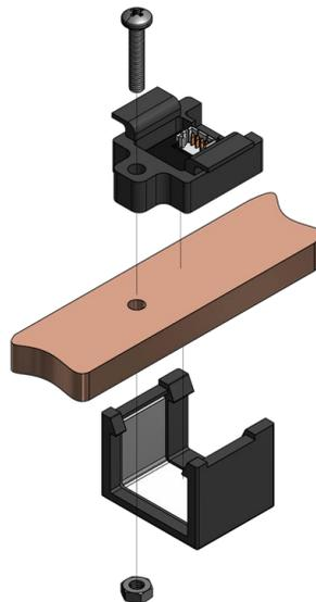
For the C version current sensor the upper half of the sensor is attached to the busbar at two points using standard hardware. The lower half of the housing is then clipped to the upper half for a secure connection. The lower housing also serves as protection for the shield.
