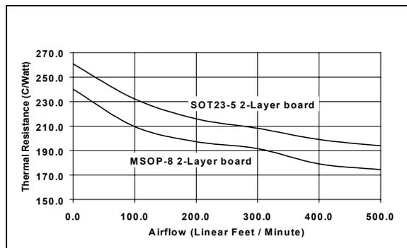
**FIGURE 8:** Thermal Resistance vs. Airflow for 2-Layer Board
