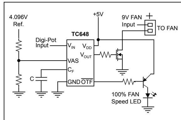
**FIGURE 7:** Fan Speed Control Circuit
