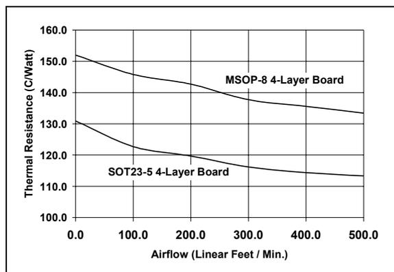
**FIGURE 9:** Thermal Resistance vs. Airflow for 4-Layer Board
