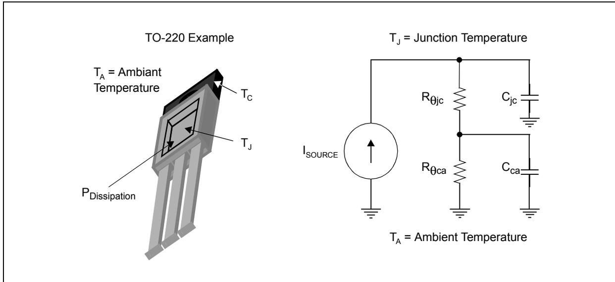
**FIGURE 1:** Analogy between Thermal Resistance and Circuit Analysis
